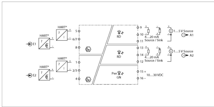
The 2-channel IMX12-AI01-2I-2IU-H0/24VDC/CC HART® isolating transducer is designed to operate intrinsically safe HART® 2-wire transducers in the Ex area and to transmit the measured signals to the non-Ex area. In addition to the analog signal also digital HART® communication signals can be transmitted bidirectionally. Alternatively, active 2-wire HART® transmitters and passive 3-wire HART® transmitters can be operated.
