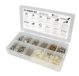
The StarTech.com PCSCREWKIT is a handy assortment of common PC fasteners for building, reparing, and maintaining computer systems. The kit includes 12 different fasteners all in a plastic carrying case with divided compartments. Includes 50 screws in each of 7 category types for a total of 350 screws as well as an assortment of standoffs.
