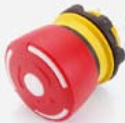
Emergency-stop non illuminated, plug-in terminals, twist release, 32 mm diameter for 22.5 mm mounting, foolproof to EN 60947-5-5
