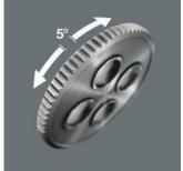
The reversible ratchet with 72 finepitched teeth has a low return angle of only 5°. This short stroke allows fast and precise work in all types of installation.
