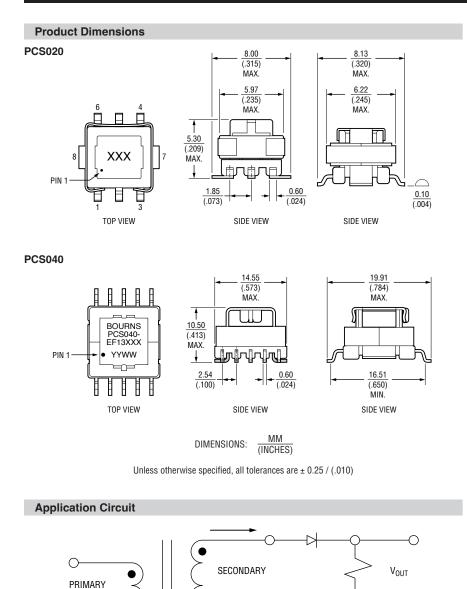
Terminating resistor  $R_T$  is based on 1 volt output with the rated current 20 amps for the PCS020 and 40 amps for the PCS040 through the Primary. The terminating resistor can be
