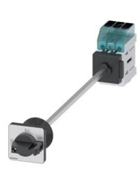
Switch disconnector 3LD3, main switch 3-polig, lu 40A operational switch at AC-23 A at 400 V 15,0 kW floor mounting Base mounting with door coupling center-hole 22,5 mm knob-operated mechanism black 48 x 48 mm
