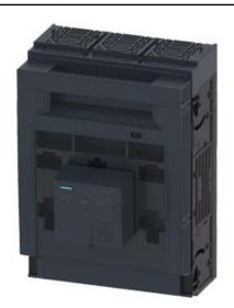
FUSE-SWITCH-DISCONNECTOR 3-POLE, NH2, 400A MOUNTING PLATE CONSTRUCTION COVER LEVEL 70 MM FLAT CONNECTOR FUSE MONITORING ELECTRONIC, EFM 10
