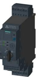
SIRIUS, COMPACT STARTER, DIRECT STARTER 690 V, 110 ... 240 V AC/DC, 50 ... 60 HZ, 1 ... 4 A, IP20, CONNECTION MAIN CIRCUIT: SPRING-LOADED TERMINAL, CONNECTION AUXILIARY CIRCUIT: SPRING-LOADED TERMINAL
