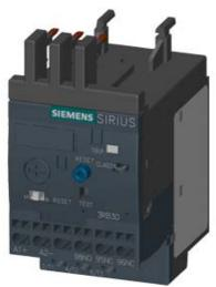
OVERLOAD RELAY 0.32...1.25 A FOR MOTOR PROTECTION SIZE S00, CLASS 20 CONTACTOR ASS. MAIN CIRCUIT: SPR.-LOAD.TERM. AUX.CIRCUIT: SPR.-LOAD.TERM. MANUAL-AUTOM.-RESET
