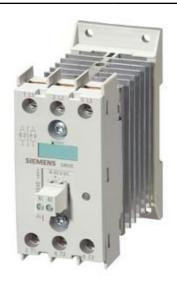
SOLID-STATE CONTACT.3PHASE 3RF2 AC51 10A 40 DEG. C 48-600V / 110V AC 2-PHASE CONTROLLED SCREW TERMINAL BLOCKING VOLTAGE 1200V
