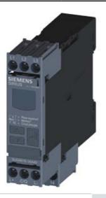
DIGITAL MONITORING RELAY FOR THREE-PHASE MAINS VOLTAGE FOR IO LINK AC 50 TO 60 HZ 3X 160 TO 690V LINE PHASE SEQUENCE, PHASE FAILURE, PHASE ASYMMETRY UNDER- AND OVERVOLTAGE HYSTERESIS 1-20V NETWORK STABILITY TIME TRIGGER DELAY TIME 1 CHANGEOVER, SCREW CONNECTION
