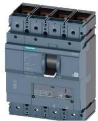
CIRCUIT BREAKER 3VA2 IEC FRAME 630 BREAKING CAPACITY CLASS C ICU=110KA @ 415 V 4-POLE, LINE PROTECTION ETU320, LI, IN=400A OVERLOAD PROTECTION IR=160A ...400A SHORT CIRCUIT PROTECTION II=12 X IN NEUTRAL PROTECTION ADJUSTABLE(OFF,50%,100%) BUSBAR CONNECTION
