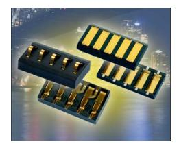
This unique battery or removable module style connector is different from most others in that it allows for the pluggable device to be swiped or connected from either direction. The spring contact offers enhanced contact deflection range over existing connectors in the market with a full 1.4mm of travel after contact engagement. This contact design allows the connector to absorb more of the plastic or housing tolerances making it more functional and reliable in real life applications.
