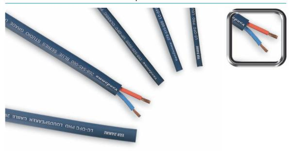
Van Damme Blue Series Studio Grade Speaker Cable caters not only for the recording studio environment but also for the rehearsal studio, live and presentation markets. All are twin-axial types and range from 0.75mm conductors for 100V line through to 6.00mm conductors for long runs of low impedance speaker signals.
