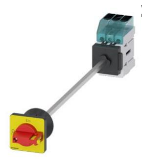
Switch disconnector 3LD3, main switch 3-polig, lu 32A operational switch at AC-23 A at 400 V 11,5 kW floor mounting Base mounting with door coupling center-hole 22,5 mm knob-operated mechanism red/yellow 48 x 48 mm
