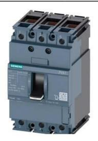
CIRCUIT BREAKER 3VA1 IEC FRAME 160 BREAKING CAPACITY CLASS N ICU=25KA @ 415 V 3-POLE, LINE PROTECTION TM210, FTFM, IN=100A OVERLOAD PROTECTION IR=100A FIXED SHORT CIRCUIT PROTECTION II=10 X IN CABLE CONNECTION
