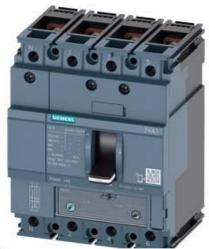
CIRCUIT BREAKER 3VA1 IEC FRAME 160 BREAKING CAPACITY CLASS H ICU=70KA @ 415 V 4-POLE, LINE PROTECTION TM240, ATAM, IN=40A OVERLOAD PROTECTION IR=28A ...40A SHORT CIRCUIT PROTECTION II=5...10 X IN NEUTRAL UNPROTECTED BUSBAR CONNECTION
