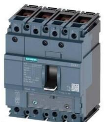
CIRCUIT BREAKER 3VA1 IEC FRAME 160 BREAKING CAPACITY CLASS H ICU=70KA @ 415 V 4-POLE, LINE PROTECTION TM240, ATAM, IN=16A OVERLOAD PROTECTION IR=11,2A ... 16A SHORT CIRCUIT PROTECTION II=5 X IN NEUTRAL PROTECTION 100% BUSBAR CONNECTION
