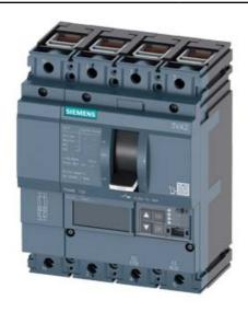
CIRCUIT BREAKER 3VA2 IEC FRAME 100 BREAKING CAPACITY CLASS C ICU=110KA @ 415 V 4POLE, LINE PROTECTION ETU560, LSIG, IN=25A OVERLOAD PROTECTION IR=10A ...25A SHORT CIRCUIT PROTECTION ISD=0,6..10X IN, II=1,5..12X IN NEUTRAL PROTECTION ADJUSTABLE (OFF, UPTO 160%) GROUNDFAULT, SWITCHABLE IG=0,2... 1 X IN, TG=0,050,8MS CABLE CONNECTION
