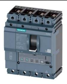
CIRCUIT BREAKER 3VA2 IEC FRAME 160 BREAKING CAPACITY CLASS H ICU=85KA @ 415 V 4POLE, LINE PROTECTION ETU330, LIG, IN=100A OVERLOAD PROTECTION IR=40A ...100A SHORT CIRCUIT PROTECTION II=1,5...12 X IN NEUTRAL PROTECTION ADJUSTABLE(OFF,50%,100%) GROUNDFAULTPROTECTION IG=0,2... 1 X IN, TG=0,1/0,3MS BUSBAR CONNECTION
