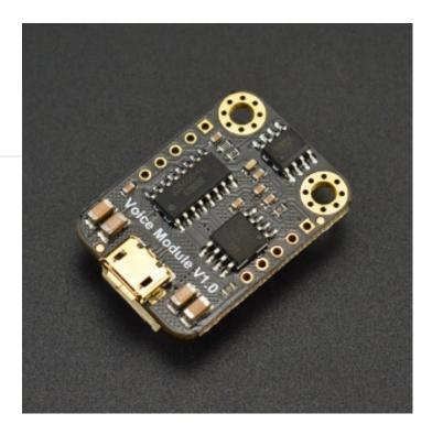
method is as simple as USB flash drive, and audios can be updated at any time. It uses the DF-Gravity interface, free from wiring; It has the ability to play the specified audio, play in loop, and adjust volume. It is suitable for all kinds of projects related to sound or voice, such as intelligent car, meteorological stations, smart home devices, vehicle navigation, toll stations, safety monitoring, machine audio navigation and so on.
