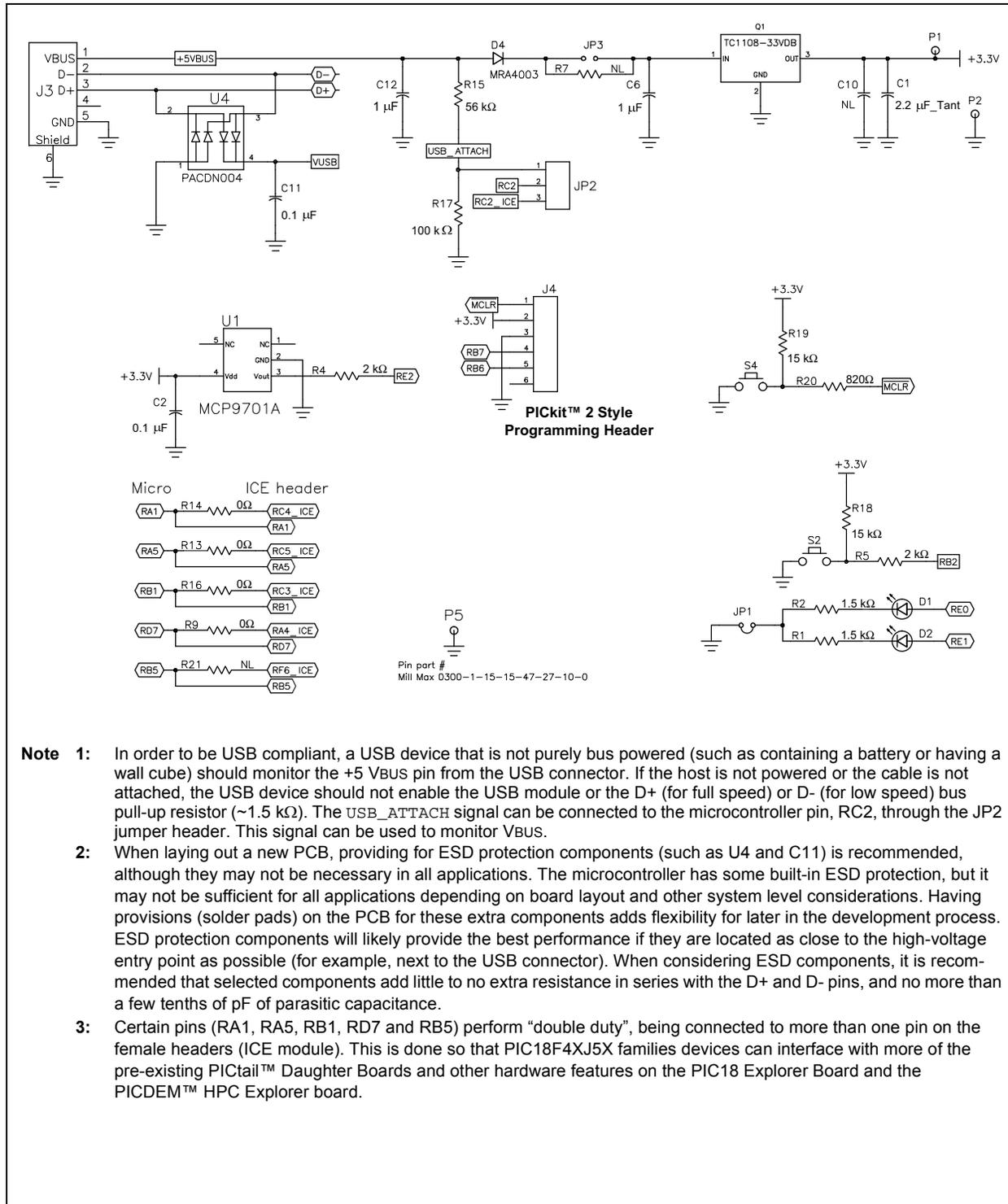
**FIGURE B-2: PIC18F4XJ5X FULL-SPEED USB DEMONSTRATION BOARD – MICROPROCESSOR<sup>(1,2)</sup>**
