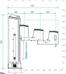
DOBOT M1 Pro is the world's first SCARA robot arm for small and medium-sized factories. Lightweight and portable, the 4-axis robot arm delivers fast setup and flexible deployment. In addition, M1 Pro's effective cost, easy programming and low maintenance make it a perfect automation solution for small & medium-sized enterprises (SMEs).
