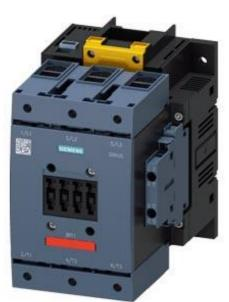
Contactor AC3: 55kW / 400 V 3-pole Size S6 Coil AC 50/60Hz and DC 200...277 V x (0,8...1,1) auxiliary contacts: 2 NO + 2 NC permanently mounted (SUVA) Main: Box terminal coil and auxilliary: screw circuit: screw terminal
