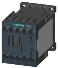
CONTACTOR, AC-3, 4KW/400V, 1NO, AC 48V, 50/60 HZ, 3-POLE, SZ S00 SCREW TERMINAL
