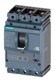
CIRCUIT BREAKER 3VA2 IEC FRAME 160 BREAKING CAPACITY CLASS L ICU=150KA @ 415 V 3POLE, LINE PROTECTION ETU350, LSI, IN=160A OVERLOAD PROTECTION IR=64A ...160A SHORT CIRCUIT PROTECTION ISD=1,5... 10 X IR, II=10 X IN BUSBAR CONNECTION
