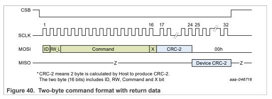
**Two-byte command:** Two-byte command format with data return.
