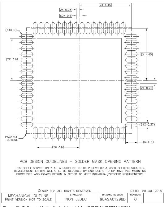
Figure 49. Reflow soldering footprint part 1 for HVQFN64 (SOT804-3(D))
