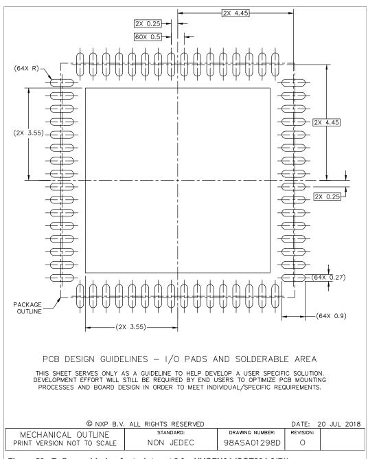
Figure 50. Reflow soldering footprint part 2 for HVQFN64 (SOT804-3(D))
