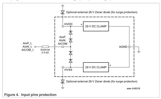
Each HV input pin is equipped with input protection diodes connected to HVDD, HVSS.
