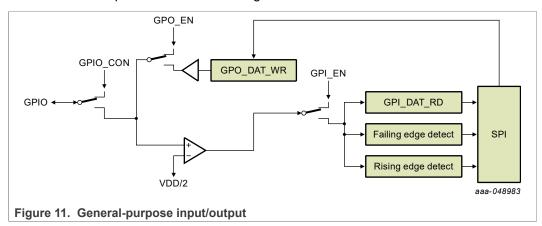
The GPIO control and data registers are organized in the following registers, right-aligned in 16-bit space:
