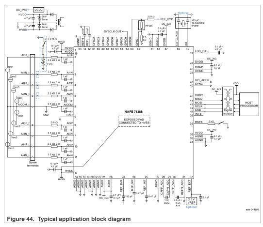
Note: Dash boxes on AI1N, AI2P, AI2N inputs represent the dashed circuitry on AI1P.
