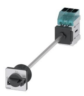
Switch disconnector 3LD3, main switch 3-polig, lu 25A operational switch at AC-23 A at 400 V 9,0 kW floor mounting Base mounting with door coupling center-hole 22,5 mm knob-operated mechanism black  $48 \times 48 \text{ mm}$
