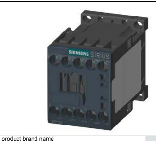
COUPLING RELAY, AC-3, 3KW/400V, 1NO, DC 24V, 0.7...1.25\*US, W. INTEGR. SUPPRESSORDIODE, SZ S00, SCREW TERMINAL
