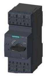
CIRCUIT-BREAKER SZ S0, FOR MOTOR PROTECTION, CLASS 10, A-REL.1.1...1.6A, N-REL.21A SPRING-L. CONNECTION STANDARD SW. CAPACITY
