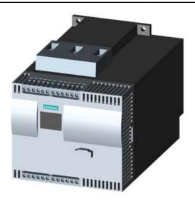
SIRIUS SOFT STARTER, VALUES WITH 575 V, 50 DEG., STANDARD: 82A, 75HP, INSIDE-DELTA CIRCUIT 3: 142A, 125HP, 400-690 V AC, 115 V AC, SCREW TERMINALS
