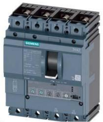
CIRCUIT BREAKER 3VA2 IEC FRAME 100 BREAKING CAPACITY CLASS L ICU=150KA @ 415 V 4POLE, LINE PROTECTION ETU350, LSI, IN=63A OVERLOAD PROTECTION IR=25A ...63A SHORT CIRCUIT PROTECTION ISD=1,5... 10 X IR, II=12 X IN NEUTRAL PROTECTION ADJUSTABLE(OFF,100%) BUSBAR CONNECTION
