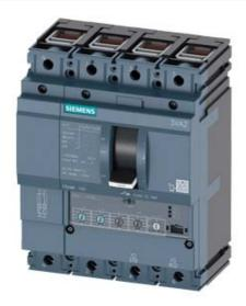
CIRCUIT BREAKER 3VA2 IEC FRAME 160 BREAKING CAPACITY CLASS C ICU=110KA @ 415 V 4POLE, LINE PROTECTION ETU350, LSI, IN=25A OVERLOAD PROTECTION IR=10A ...25A SHORT CIRCUIT PROTECTION ISD=1,5... 10 X IR, II=12 X IN NEUTRAL PROTECTION ADJUSTABLE(OFF,100%) CABLE CONNECTION
