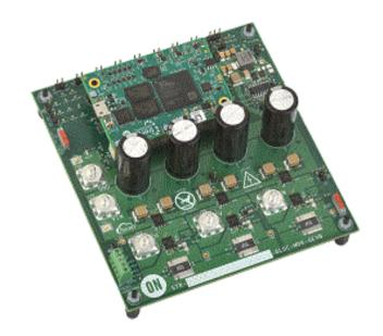
motor driver. As part of the motor development kit, the power board is compatible with the power Universal controller board enabling high-end control strategies and Al capabilities for industrial motor control. The complete kit is Strata enabled and the graphical user interface can be used to set control parameters for the motor drive.
