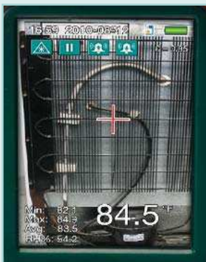
Large 2.2" color video LCD displays measurement area with temperature/humidity, min/max/avg, date, and time stamp
