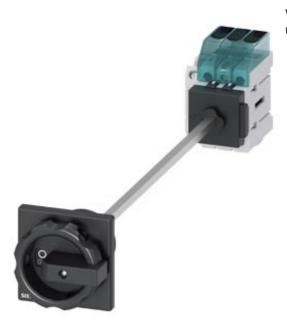
Switch disconnector 3LD3, main switch 3-polig, lu 40A operational switch at AC-23 A at 400 V 15,0 kW floor mounting Base mounting with door coupling center-hole 22,5 mm rotary operationg mechanism black 66 x66 mm with auxiliary 1NO+1NC
