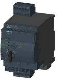
SIRIUS, COMPACT STARTER, REVERSING STARTER . 400 V, 24 V DC, 8 ... 32 A, IP20, CONN. MAIN CIRCUIT: SPRING-LOADED TERMINAL, CONN. CONTROL CIRCUIT: SPRING-LOADED TERMINAL
