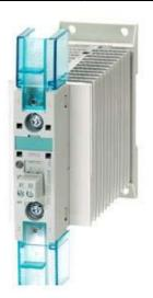
SEMI-COND. CONTACTOR 3RF2,1-PH. AC 51 30 A 40 DEGREES C 48-600 V / 24 V DC RING TERMINAL
