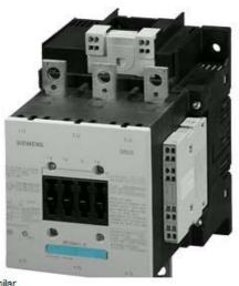
CONTACTOR, 90KW/400V/AC-3 AC(40...60HZ)/DC OPERATION UC 440-480V AUXILIARY CONTACTS 2NO+2NC 3-POLE, SIZE S6 BAR CONNECTIONS CONVENT. OPERATING MECHANISM CAGE CLAMP TERMINAL
