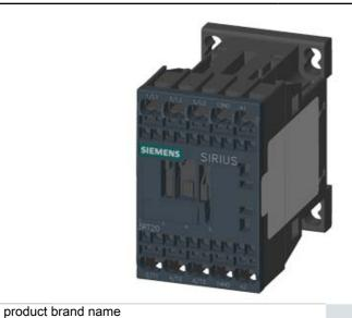
CONTACTOR, AC-3, 7.5KW/400V, 1NO, AC 42V, 50/60 HZ, 3-POLE, SZ S00 SPRING-LOADED TERMINAL
