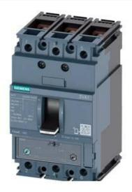
CIRCUIT BREAKER 3VA1 IEC FRAME 160 BREAKING CAPACITY CLASS S ICU=36KA @ 415 V 3-POLE, LINE PROTECTION TM240, ATAM, IN=20A OVERLOAD PROTECTION IR=14A ...20A SHORT CIRCUIT PROTECTION II=8...16 X IN BUSBAR CONNECTION
