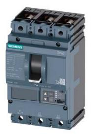
CIRCUIT BREAKER 3VA2 IEC FRAME 160 BREAKING CAPACITY CLASS C ICU=110KA @ 415 V 3POLE, LINE PROTECTION ETU550, LSI, IN=25A OVERLOAD PROTECTION IR=10A ...25A SHORT CIRCUIT PROTECTION ISD=0,6..10X IN, II=1,5..12X IN NEUTRAL PROTECTION OPTIONAL WITH EXT. CT,UPTO 160% BUSBAR CONNECTION
