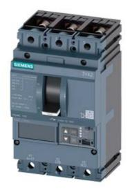
CIRCUIT BREAKER 3VA2 IEC FRAME 160 BREAKING CAPACITY CLASS M ICU=55KA @ 415 V 3POLE, LINE PROTECTION ETU550, LSI, IN=63A OVERLOAD PROTECTION IR=25A ...63A SHORT CIRCUIT PROTECTION ISD=0,6..10X IN, II=1,5..12X IN NEUTRAL PROTECTION OPTIONAL WITH EXT. CT,UPTO 160% BUSBAR CONNECTION
