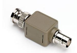
The TA051 feed-through attenuator is a coaxial terminator with BNC connectors. It is useful for connecting signals from 50  $\Omega$  sources into instruments with 1 M $\Omega$  impedance inputs, such as oscilloscopes.
