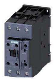
CONTACTOR,AC3:30KW/400V, 1NO+1NC, 48 - 80V AC/DC, WITH VARISTOR, 3-POLE, SIZE S2, SCREW TERMINAL
