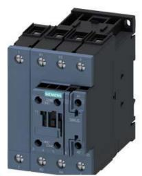
2NO+2NC CONTACTOR,AC3:18.5KW 20-33V AC/DC,VARISTOR, 4-POLE, 2NO+2NC, SIZE S2, SCREW TERMINAL 1NO+1NC INTEGRATED
