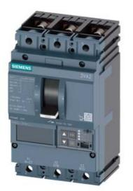
CIRCUIT BREAKER 3VA2 IEC FRAME 250 BREAKING CAPACITY CLASS C ICU=110KA @ 415 V 3POLE, LINE PROTECTION ETU550, LSI, IN=250A OVERLOAD PROTECTION IR=100A ...250A SHORT CIRCUIT PROTECTION ISD=0,6..10X IN, II=1,5..10X IN NEUTRAL PROTECTION OPTIONAL WITH EXT. CT,UPTO 160% BUSBAR CONNECTION
