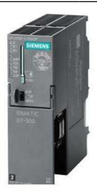
SIMATIC S7-300 CPU315F-2 PN/DP, CENTRAL PROCESSING UNIT WITH 512 KBYTE WORKING MEMORY, 1. INTERFACE MPI/DP 12MBIT/S, 2. INTERFACE ETHERNET PROFINET, WITH 2 PORT SWITCH, MICRO MEMORY CARD NECESSARY
