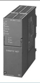
SIMATIC NET, CP 343-1 LEAN COMMUNICATION PROCESSOR FOR CONNECTING SIMATIC S7-300 TO IND. ETHERNET VIA TCP/IP AND UDP, MULTICAST, SEND/RECEIVE W/ AND W/O RFC1006, FETCH/ WRITE, S7-COMMUNICATION(SERVER) PROFINET IO-DEVICE INTEGRATED 2-PORT SWITCH ERTEC 200, BG EXCHANGE W/O PG, SNMP DIAGNOSTICS, INITIALIZATION VIA LAN, 2 X RJ45 CONNECTION FOR LAN WITH 10/100 MBIT/S
