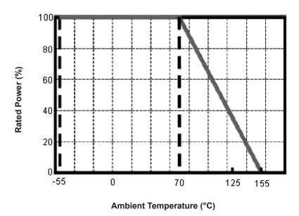
Max. dissipation in percentage of rated power as a function of the ambient temperature
