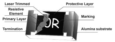
Construction of a Chip-R
